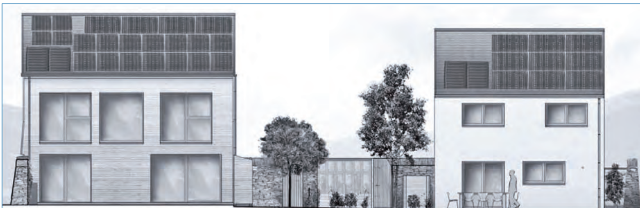
Figure 2: These design drawings show Larch House’s much higher glazing area (55% of the south side), compared to Lime House’s 20% glazing ratio.
